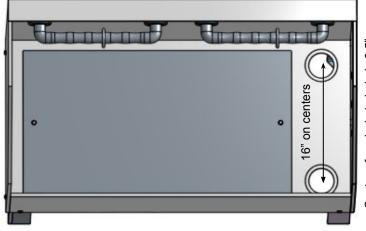
Center of each drain hole is 3.5" from inside of front/back wall
